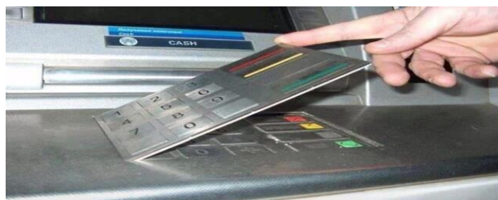
Fake Keypad to capture PIN
