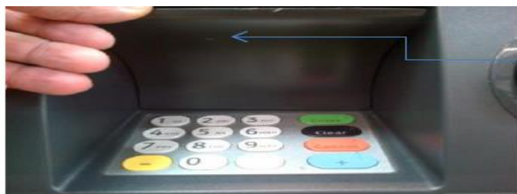
Fake Keypad to capture PIN
